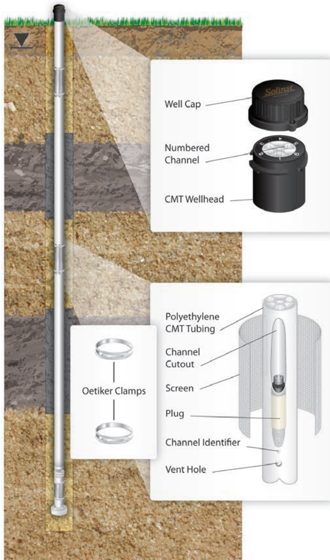
Typical 3 or 7-Channel CMT Installation using layers of bentonite and sand backfilled from surface.
